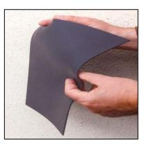
MAS-200 series are thin, flexible resonant absorbers which are available for frequencies within the 0.9 GHz to 16.0 GHz frequencies range. Center frequency absorption is approximately -25 dB and bandwidth is typically 10%. Product is formulated using custom magnetic active fillers.
