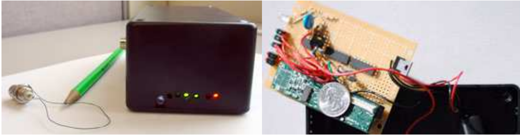
Fig. 1. Our assembled PICCAL credit card emulator
