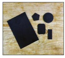
MWT'S MAS-310 thin flexible urethane MagRAM absorber designed for use over the range of 0.01 to 16 GHz (which covers all the RFID frequencies of 125 KHz through 13.56 MHz).
