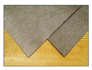
ME-2100 is a simple solution for effective RF signal attenuation in many commercial applications. It provides -100 dB RF isolation from 100 MHz to 1 GHz and more than -70 dB to 18GHz. Very light, thin, flexible, wear and tear resistant, it can be applied directly to studs, standard sheetrock and other materials using simple and inexpensive methods.
