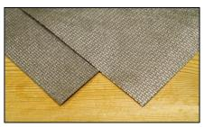
ME-2100 is a simple solution for effective RF signal attenuation in many commercial applications. It provides <u>-100 dB RF isolation</u> from 100 MHz to 1 GHz and more than -70 dB to 18GHz. Very light, thin, flexible, wear and tear resistant, it can be applied directly to studs, standard sheetrock and other structures using simple and inexpensive methods. The product is well suited to both new and retrofit construction. It provides a good degree of
