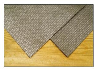
ME-2100 is a simple solution for effective RF signal attenuation in many commercial applications. It provides <u>-100 dB RF isolation from 100 MHz to 1 GHz and more than -70 dB to 18GHz.</u> Very light, thin, flexible, wear and tear resistant, it can be applied directly to studs, standard sheetrock and other materials using simple and inexpensive methods.
