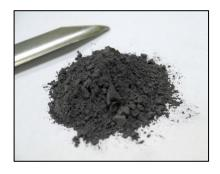
MF-401 Type S powder is an Iron Silicide product providing low corrosion, high temperature and high magnetic saturation properties. It has enhanced electromagnetic properties in comparison with Iron aluminide, yet retains significant anti corrosion and elevated temperature properties. With a nominal Curie point above Carbonyl Iron Powder, this product will perform day in and day out in high heat flux and aggressive environmental conditions.
