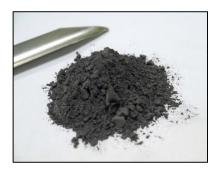
MF-402 Type CR powder is an Iron Chrome silicide product providing low corrosion, high temperature and high magnetic saturation properties. It has enhanced electromagnetic properties in comparison with Iron silicide and Iron aluminide, yet retains significant anti corrosion and elevated temperature properties. With a nominal Curie point similar to Carbonyl Iron Powder, this product will perform day in and day out in high heat flux and aggressive environmental conditions.
